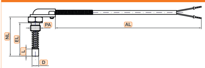
5: Bent protection tube and loose threaded connection with spring
