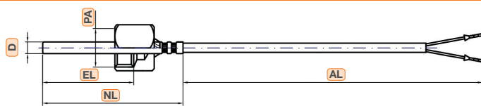
3: Protection tube with fixed internal thread
