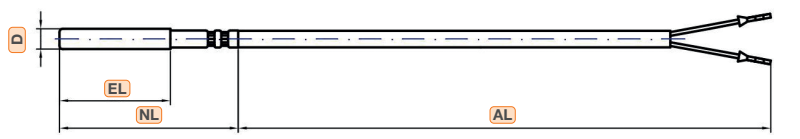
2: Extended protection tube (D = 8 mm)
