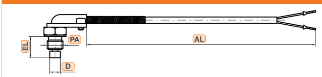
3: Bent protection tube and loose threaded connection with spring
