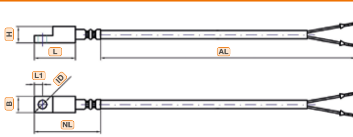
Cable temperature probe with metal surface cube and mounting hole (Construction 3)
