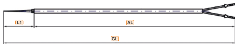
Thermocouple with exposed hot junction (Construction 3)
