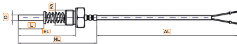
Stepped protection tube, loose external thread and spring
