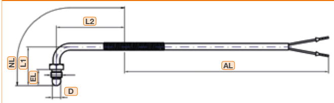
Protection tube and multiparts angle connector, loose threaded connection
