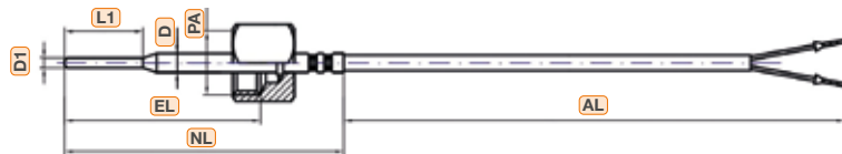
Straight protection tube, loose external thread and spring
