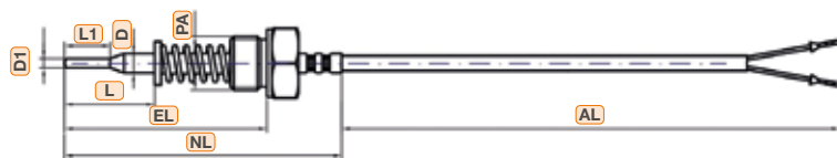
Straight protection tube, loose internal thread and spring
