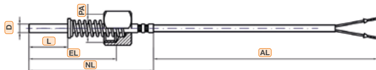
Stepped protection tube, loose internal thread and spring
