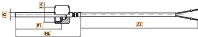
Stepped protection tube and loose internal thread
