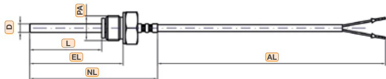
Stepped protection tube and loose external thread
