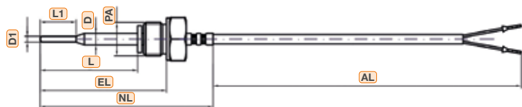
Straight protection tube and loose internal thread
