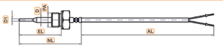
Stepped protection tube with fixed external thread
