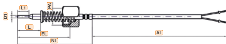
Stepped protection tube, loose internal thread and spring
