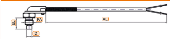
Bent protection tube and loose threaded connection with spring
